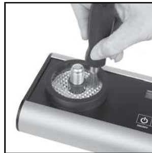
Figure 7. Cleaning the cell.
